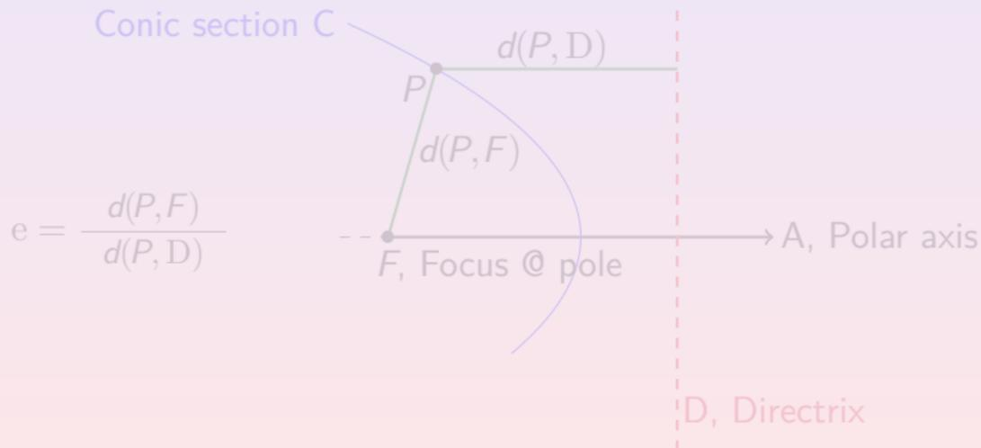
Figure 8: Polar representation of conic sections
