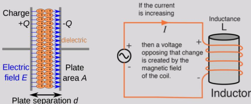
Figure 3: Left: capacitor, Right: inductance
