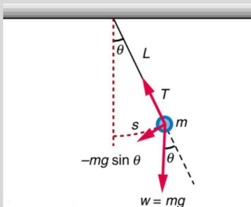
Figure 5: A simple pendulum system
