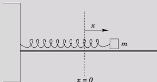
Figure 1: The spring-mass system
