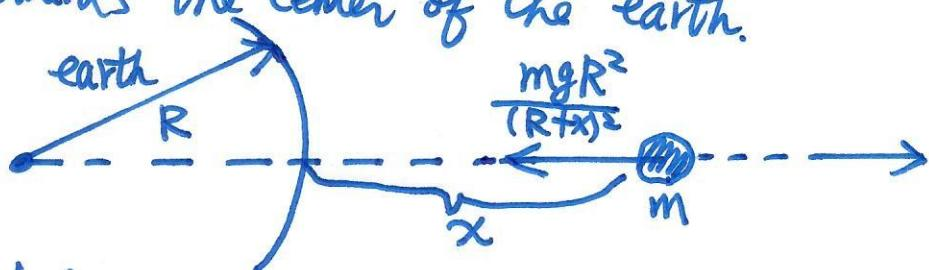
A body of constant mass  $m$  is projected from the earth in a direction perpendicular to the earth's surface with an initial velocity  $v_0$ . Assuming that there is no air resistance, prove: (1) The maximum altitude  $A_{\max} = \frac{v_0^2 R}{2gR - v_0^2}$
