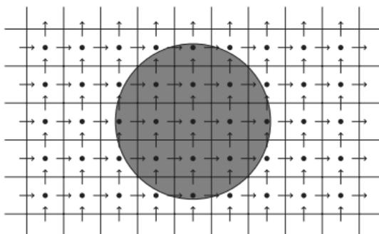
*Diagram of the computational domain  $\Omega$  with staggered grid, where the unknowns  $u$ ,  $v$  and  $p$  are approximated at the grid points marked by  $\rightarrow$ ,  $\uparrow$  and  $\bullet$ , respectively*
