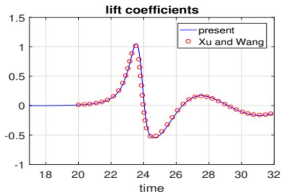
*The time evolution of drag and lift coefficients,  $C_d$  and  $C_l$ , for the upper cylinder in the flow around two cylinders compared with the results of Xu-Wang (JCP 2006)*
